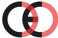
False CE Mark (too close)
