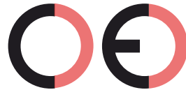
False CE Mark (too far)
